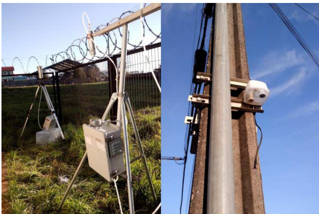
Figure 3.3.3. Impactors (left) and diffusive samplers (right) used to monitor PM and gas concentrations.
