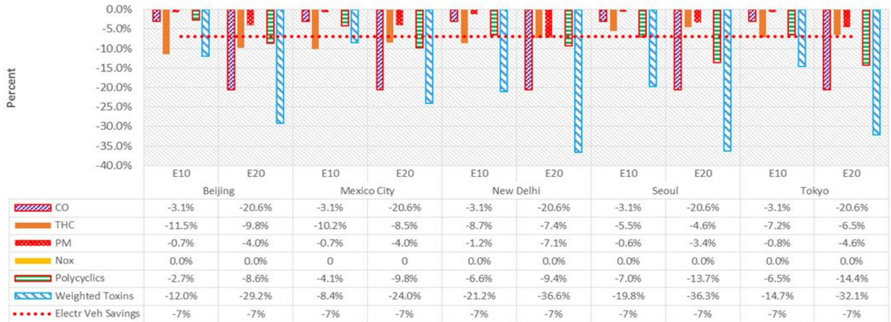
iBEAM Emissions Results by City and Ethanol Blend (7% EV, 50% GDI Share by 2027)
