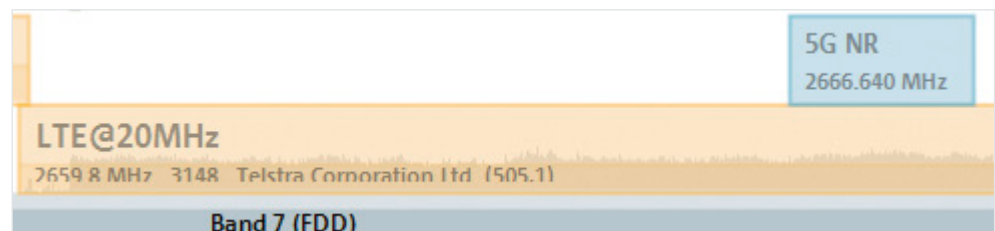
Fig. 2: Dynamic spectrum sharing, overlapping LTE and 5G NR carrier in the frequency domain
