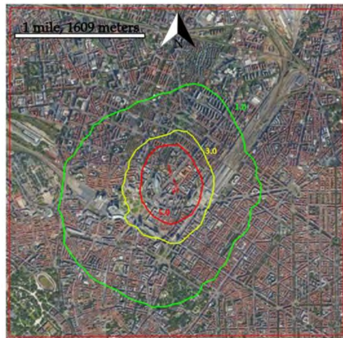
Figure 2. Example of a map resulting from atmospheric dispersion simulations representing the iso-concentration lines corresponding to the 98th percentile of the odour concentration values of 1, 3, and 5 \text{ouE}\cdot\text{m}^{-3} .
