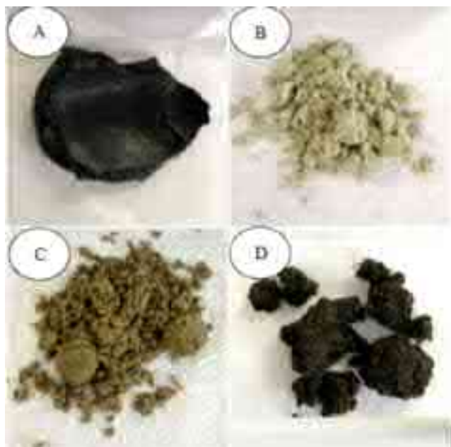
Figure 2: Wastes of Kraft process: A - dregs, B - lime mud, C - grits, and D - pulp mill sludge.
