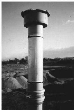
(a) DustScan directional monitoring equipment developed
