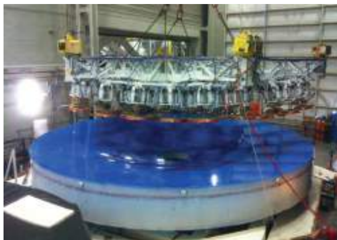
Figure 4. Left: Artist conception of the LSST, viewed from the telescope platform. Right: The primary-tertiary mirror combination, polished to specifications and ready to be stored. © LSST, licensed under CC BY-SA 4.0.
